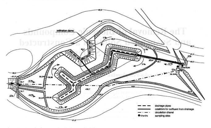
Fig. 1. The schematic of constructed wetland system in Bielkowo.
